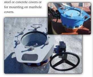
**Foam Separators** are made of stainless steel with internal baffling and fine water spray nozzles to separate the foam from the take-off gas, to help protect pressure/vacuum relief valves and flame arresters and other gas safety and utilization equipment.
