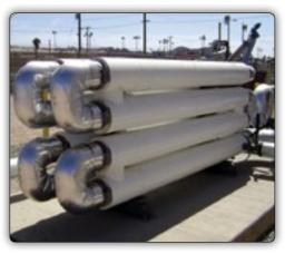
**Custom concentric tube units** have been designed with 4" to 14" sludge tubes. The concentric tube units are configured with the sludge tubes enclosed by hot water tubes. Sludge is pumped through the inner tube while hot water is pumped through the outer tube. Heat transfer takes place across the sludge tube wall. ASME certification is available.
